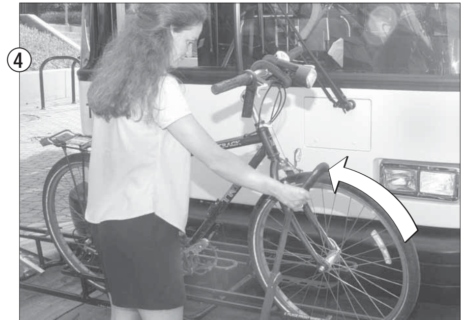
4 Secure the bike by lifting the bar up and clamping it over the tire.
