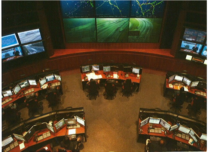
GDOT is using remote communications to actively manage traffic signals from the Transportation Management Center.
